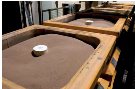
Figure 100: Molded cluster in quartz sand (6-cylinder heads of the company BMW GROUP (COPYRIGHT))
