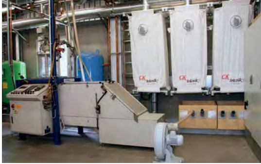
Figure 130: Batch pre-expander PRO-A-500 of the company STYROLOGIC at the FRAUNHOFER IFAM (COPYRIGHT) in Bremen
