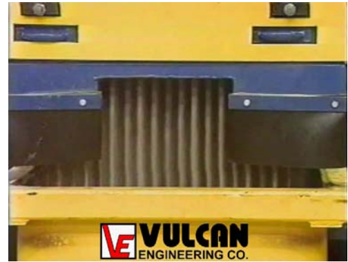
Sand Rain Gate
