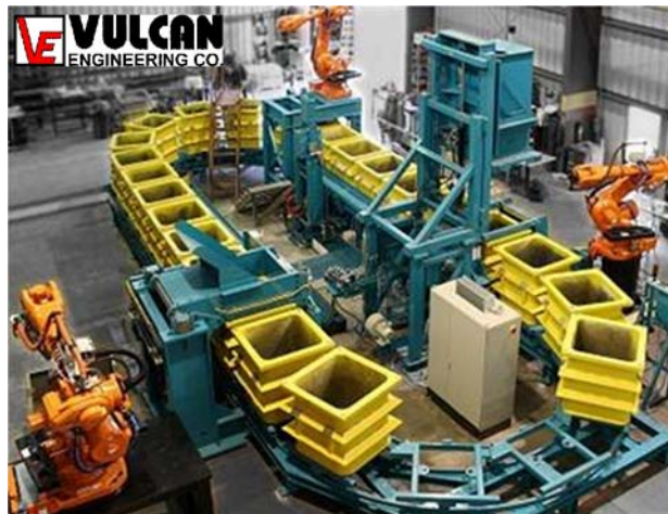
30 FPH Aluminum Lost Foam Line w/25 Minutes Cooling Note the Robots for Insertion of Foam/Pouring & Extraction
